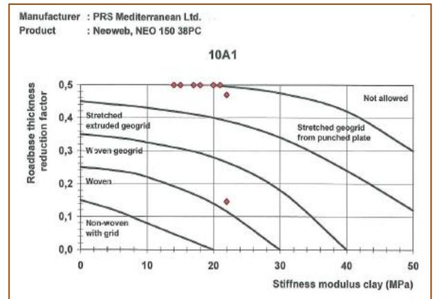
Figure 2. Roadbase Reduction Factor for PRS-Neoweb (limited)
