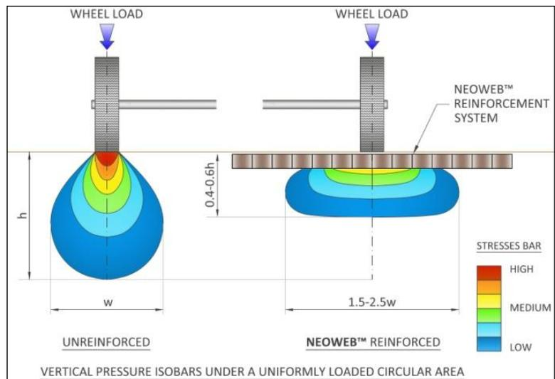
These benefits decrease the amount of excavation, hauling, and aggregate placement and compaction resulting in significant economic and environmental gains. Reinforcement with PRS-Neoweb also increases the service life of pavement structures, thereby reducing their operational and maintenance cost requirements. This enables transportation management professionals to allocate the budgets from maintenance and repair to the construction of new roads and infrastructure.
