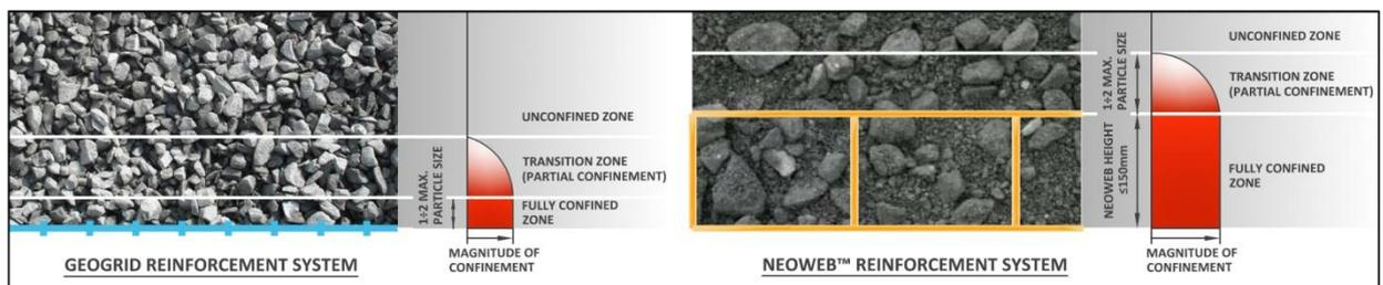
The PRS-Neoweb fully confined zone is equivalent to the height of the cell. In addition the particle size is limited to 1/3 of the cell diameter, which is many times larger than geogrid apertures.
